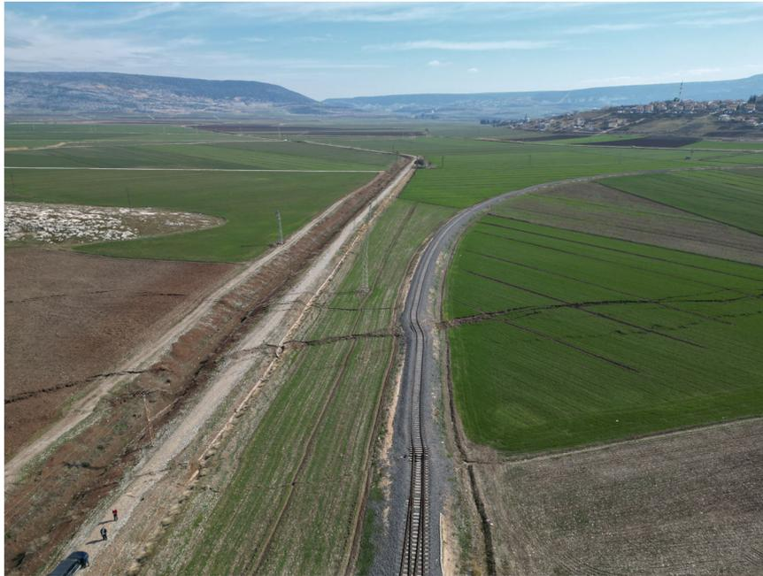
**Fig. 1 Distributed surface faulting caused by the 2023 Kahramanmaraş Earthquake Sequence.** Offset roads, railroad tracks and farm fields near the epicenter of the M7.8. Photo by Sinan Akciz, California State University, Fullerton.
