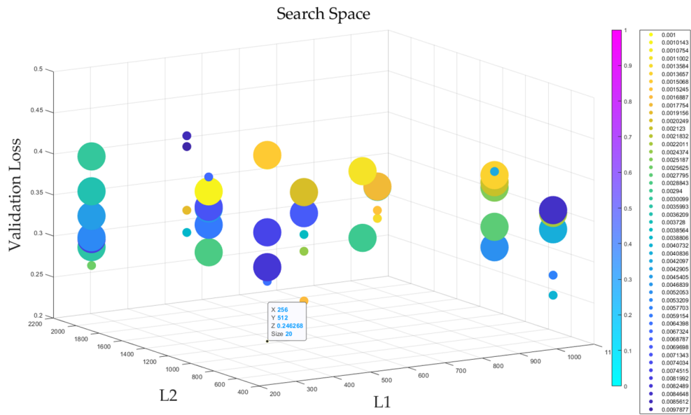
Figure 4. Visualization of hyperparameter space search results of AutoMPDNN. The horizontal axis X represents l_1 , the vertical axis Y represents l_2 , and the Z-axis represents the automated evaluation of validation loss. Each search result is denoted by a circle, with different colors indicating various learning rates, and the circle's size represents the batchsize .
