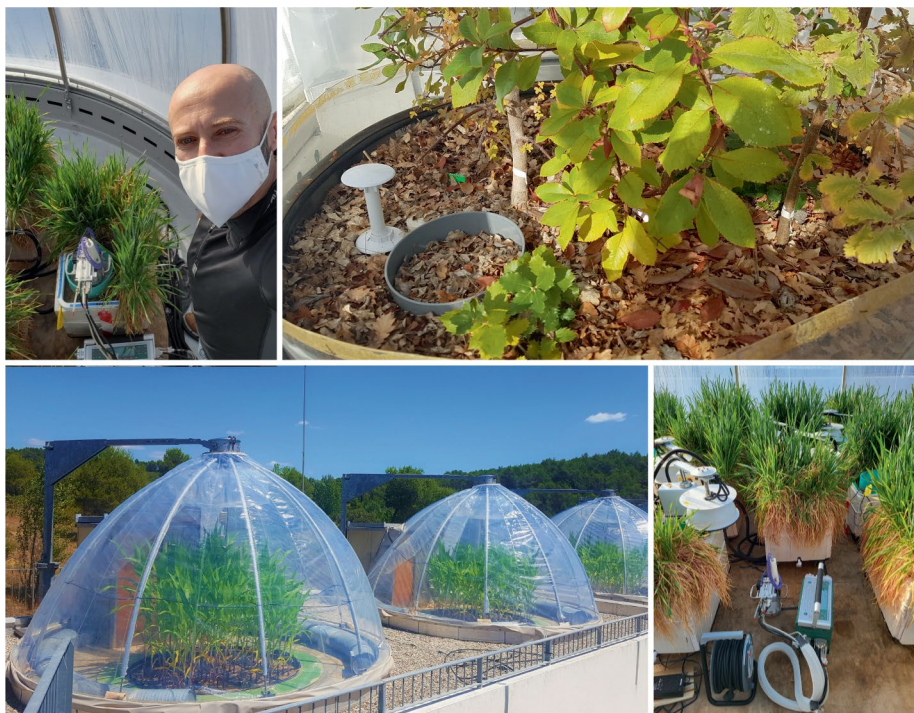
Alexandru Milcu (upper left) directs the European Ecotron of Montpellier. Scientists can do various types of experiments in the controlled environments that micro-, meso- and macrocosms provide. All units have automated measurement of gases from soil. One project underway is to compare the carbon sequestration effects of adding of biochar or basalt to soil.
