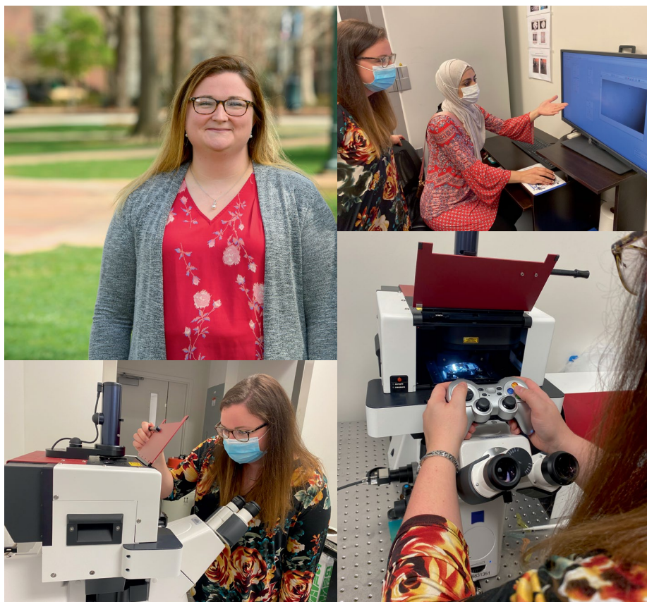
In her lab, Nikki Reinemann (top left), graduate student Omayma Al Azzam and the rest of the team combine fluorescence microscopy with high-resolution optical trapping, in which a laser beam is used to measure the forces that cytoskeletal proteins generate.
