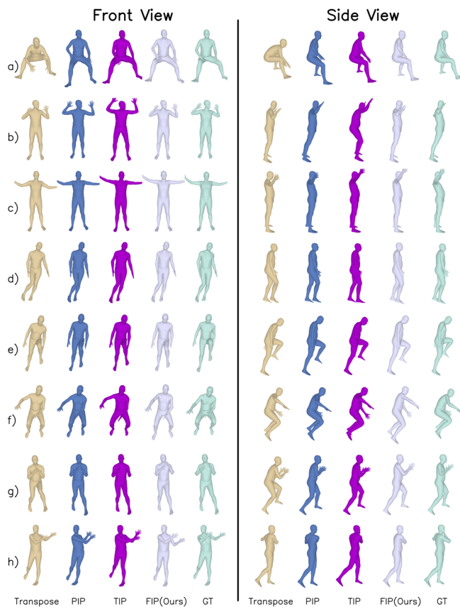
Fig. 3 | Motion reconstruction of different methods. Panels (a)–(h) represent some actions selected from the test set. The yellow color represents the reconstruction results obtained from Transpose, the blue color represents the reconstruction results obtained from Physical Inertial Poser (PIP), the purple color represents the reconstruction results obtained from Transformer Inertial Poser (TIP), the white color represents the reconstruction results obtained from Fast Inertial Poser (FIP), and the green color represents the Ground Truth (GT).
