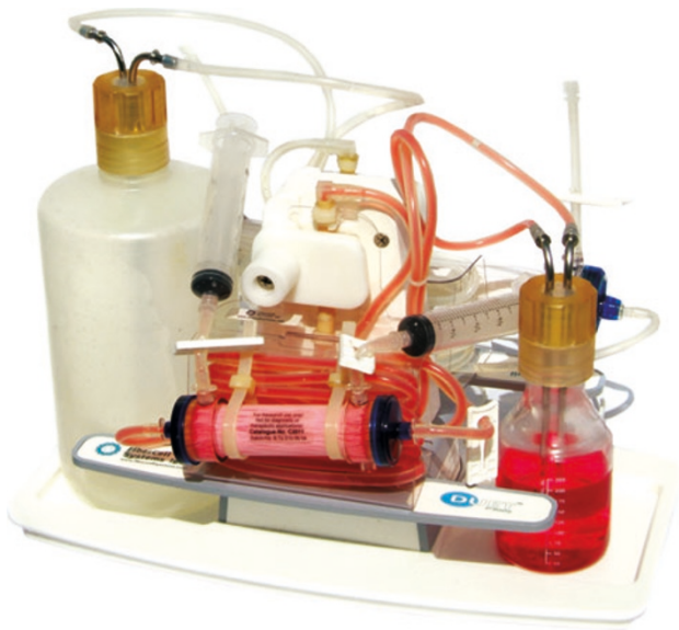
The Duet pump system from FiberCell Systems can support up to two hollow-fiber culture cartridges simultaneously. (Courtesy of FiberCell Systems.)
