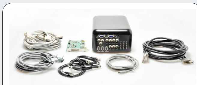
Figure 2 | The Nikon NI-BB kit provides NIDAQ connections to various hardware devices for direct-triggered control by means of direct cable connections to predefined connectors, making software setup of devices and NIDAQ channels simple
