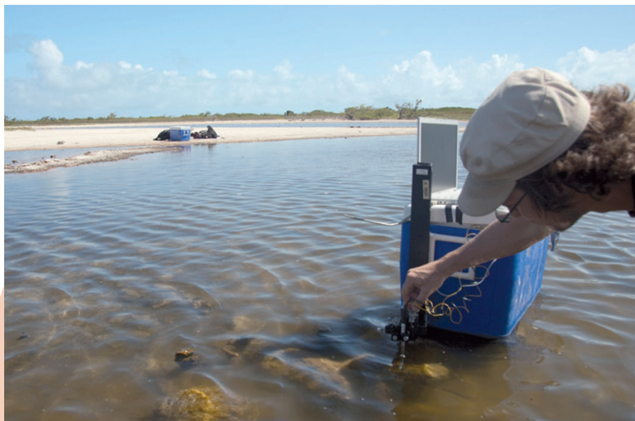
Makeshift floating microsensor, with Stefan Lalonde trying to find ways to keep the device stable while measuring underwater gas profiles.
