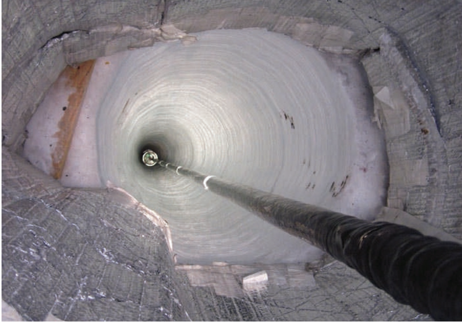
One of the detectors of the neutrino 'telescope' is lowered into place.
